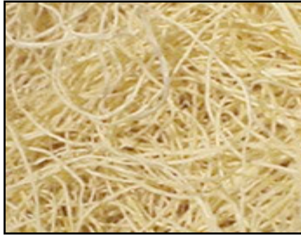
Wood excelsior fiber close-up (Source: Wholesale Supplies,
