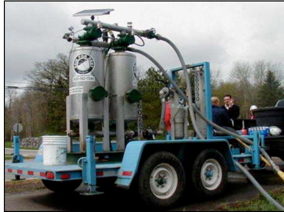
Sand Media Particulate Filter
